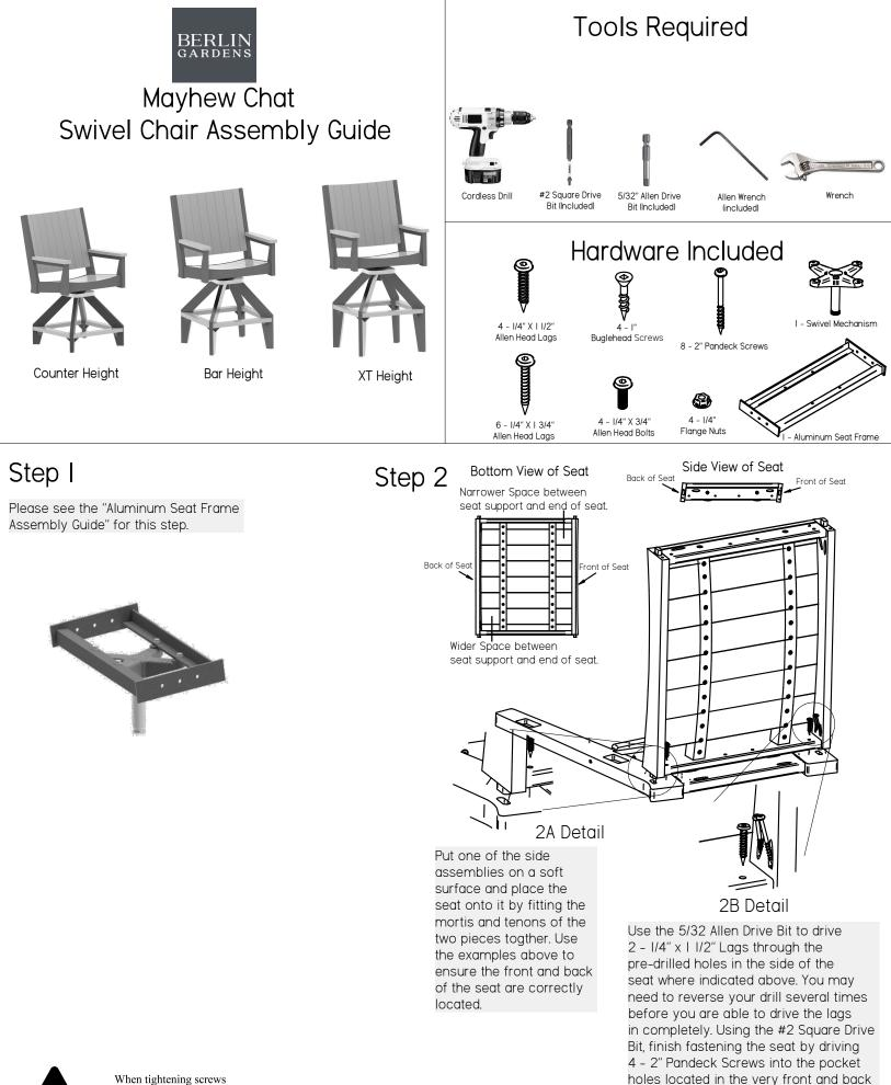
When tightening screws or lags, **DO NOT OVER-TIGHTEN** to avoid stripping their hold on the material!
